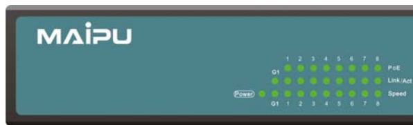
Figure 1-14 MyPower S3008G-POE LED layout
