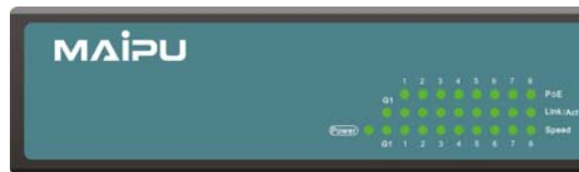
Figure 1-12 MyPower S3008G-POE LED layout
