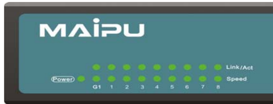
Figure 1-11 MYPower S3008G LED layout
