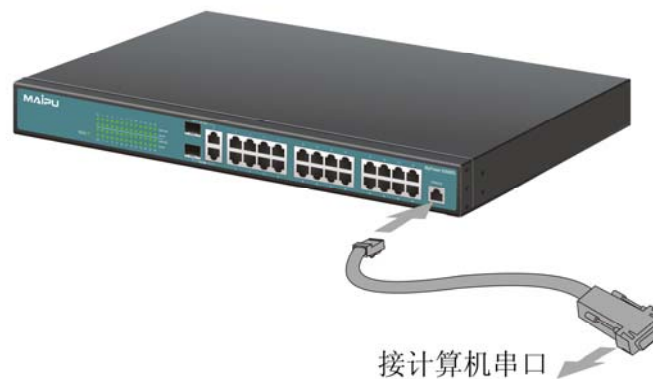
Figure 2-3 Connecting Console to MyPower S3000
