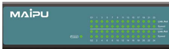
Figure 1-10 MyPower S3026G-M LED layout
